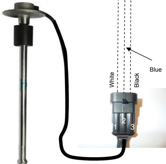
Pin 1 - Wh - Low Fuel Warning Pin 2 - Bl - Output signal Pin 3 - Bk - Negative
