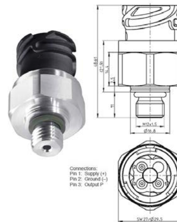
Electronic pressure sensor with voltage output.
